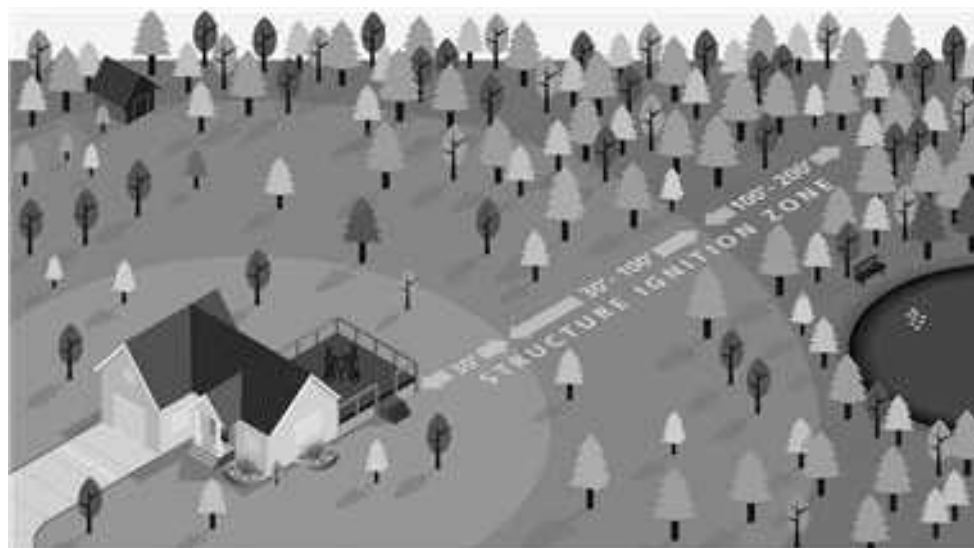
Δ FIGURE A.17.1.8 The Structure Ignition Zone. (Source: Firewise Communities Program.) [1140:Figure A.24.3.4]
